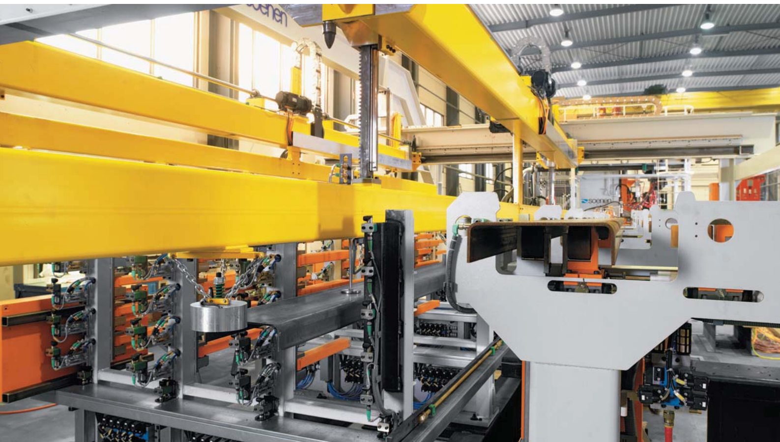
▲ In this machine holes are drilled in the carrier profiles for utility vehicle chassis.
