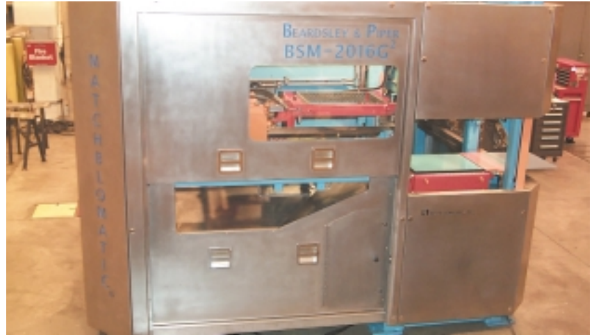
The BSM 2016G" autoomatic matchplate molding machine features advanced drive and control equipment from Rexroth.
