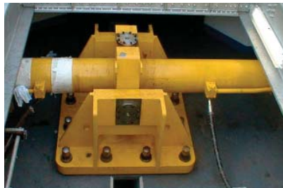
The hydraulic cylinder is mounted to the cardanic ring, which was designed to adapt to the existing footprint.
