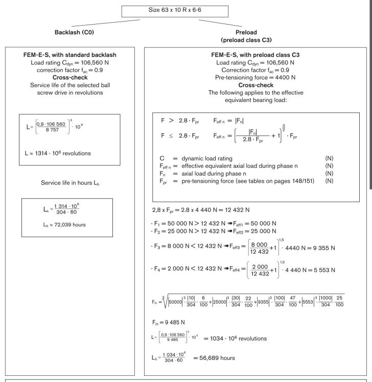
The service life of both BASAs (with standard backlash C0/with preload class C3) exceeds the required service life of 40,000 x 60% = 24,000 hours. This means that it is possible to choose a smaller BASA, subject to a review of it being undertaken.
