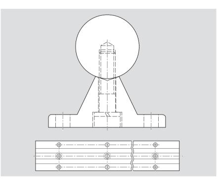
See Section "Steel shafts with ready-mounted shaft support rails" for matching shaft support rails. Precision steel shafts
