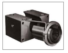
Place the mounting ring<sup>1)</sup> on as shown in the figure and use the adjusting screw to compress the radial linear bushing until it can be easily inserted into the housing bore by hand. The mounting ring hole must be about 0.5 mm larger than the outer diameter D of the radial linear bushing.
