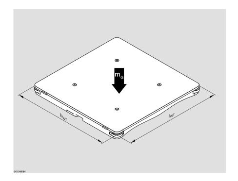
The carrying force per roller is 50 kg, and the WT must always be on at least 3 rollers. The resulting load limits for the longitudinal conveyor are illustrated in the graphic.
