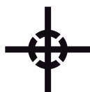
Fig. 1: Symbol for marking the center of gravity
