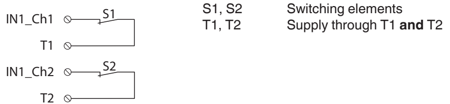
Fig. 8-11 Two-channel equivalent assignment of inputs, supply through T1 and T2 (both clocked)
