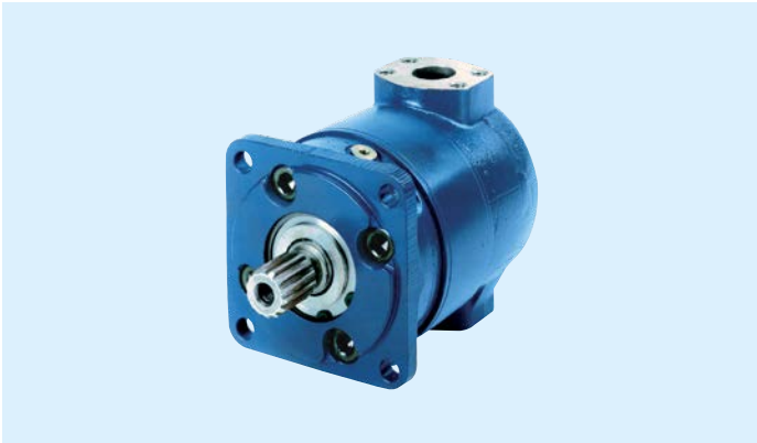
▲ MV015 – 2000 rpm, 509 lb-ft (690 Nm) Offered in single, two-speed, double output shafts, wheel-bearing style, and retractable shafts along with splined, tapered, or straight keyed shafts. Through-hole and thrust bearing options also available. SAE C mount.
