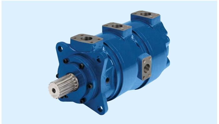
▲ MV037/057 4-Port – 500 rpm, 6032 lb-ft(8178 Nm) Combines any two displacements from the 37 and/or 57 series displacement choices in a 4-port configuration. Allows for 2- or 3-speed operation using external valving. Available in both A and D designs. Many of the same optional choices listed above are available.
