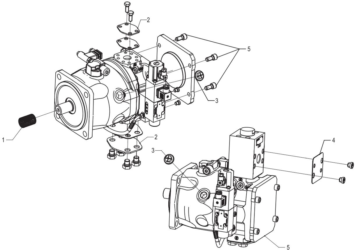
Fig. 1: Control system SYDFE1-3X
