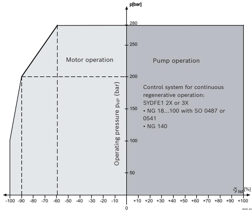
Fig. 8: Operating limits for series SYDFE1-2X and SYDFE1-3X with special rotary group for continuous regenerative operation
