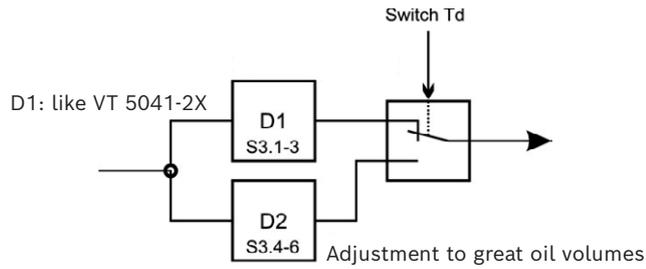
Fig. 33: Adjustment to the connected oil volume
