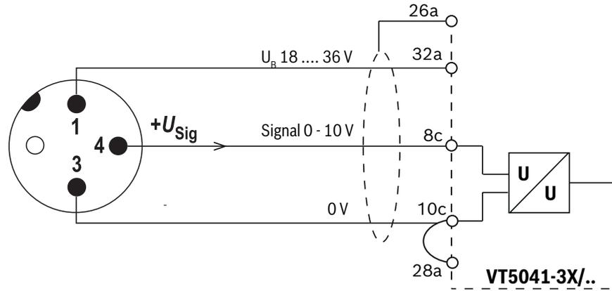
Fig. 24: Connection pattern for pressure transducer HM20...H...
