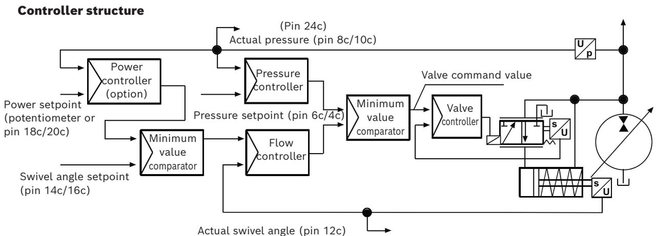
Fig. 4: Controller structure
