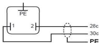
Fig. 31: Connection of the proportional valve solenoid
