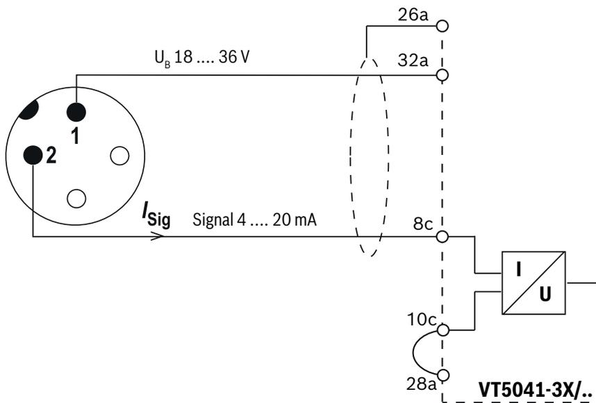
Fig. 23: Connection pattern for pressure transducer HM20...C...
