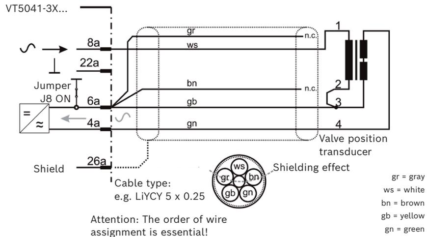
Fig. 26: Cabling for cable lengths up to 50 m
