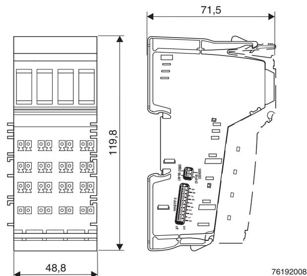
Fig. 3-2 Housing dimensions (in mm)
