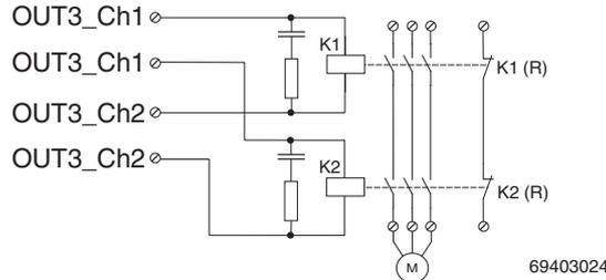
Fig. 7-7 Two-channel assignment of positive and negative switching outputs
