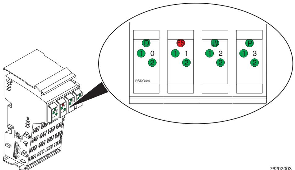
Fig. 3-3 Local diagnostic and status indicators on the R-IB IL 24 PSDO 4/4-PAC module
