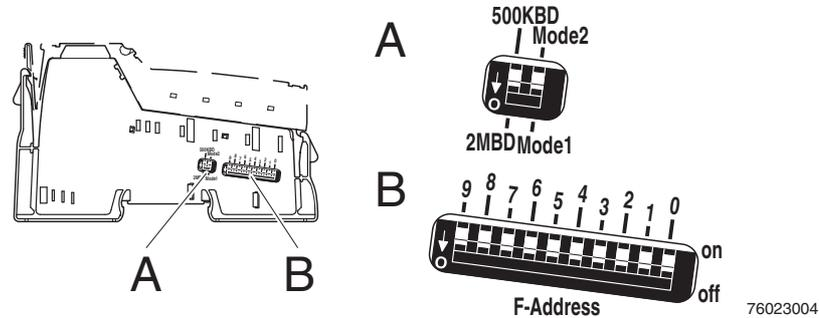
Fig. 5-1 DIP switches
