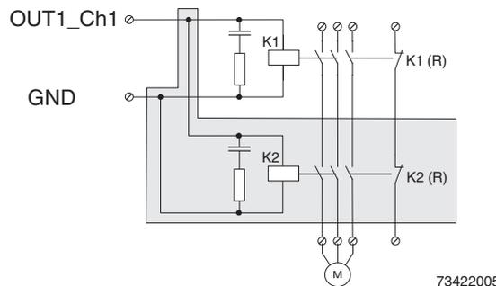
Fig. 7-5 Single-channel assignment of positive switching outputs
