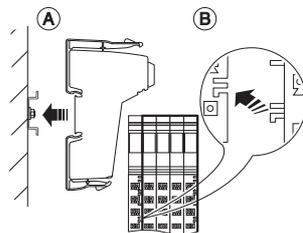
Fig. 5-3 Snapping on the safety module base
