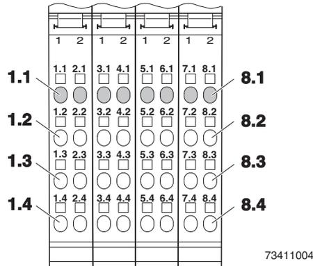
Fig. 4-2 Terminal point assignment
