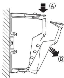
Fig. 5-5 Removing the connector
