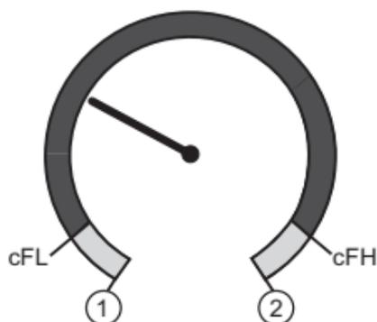
Measured value between cFL and cFH; display = red
