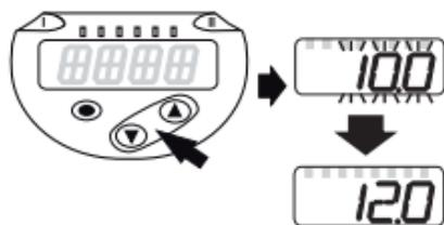
Numerical values are continuously incremented with [▲] or decremented with [▼].
