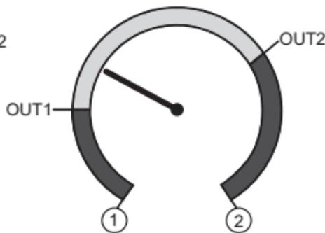
Measured value between OUT1 and OUT2; display = red
