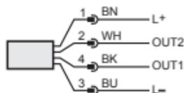
OUT1      Switching output or IO-Link
