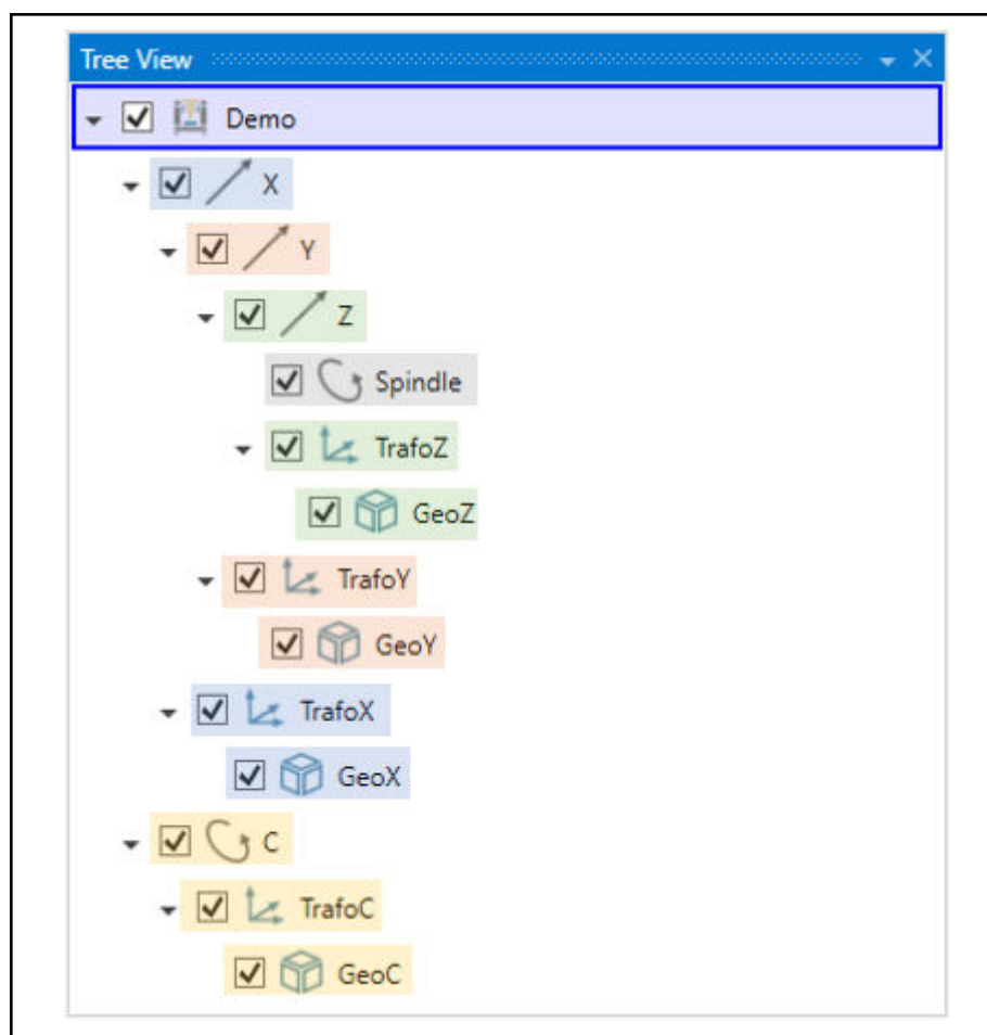
Fig. 12-6: Kinematic structure with transformation and geometry node
