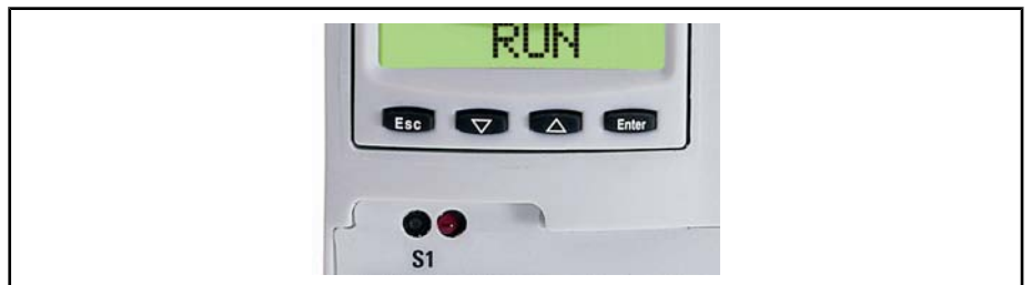
Fig. 7-3: Stop LED and recessed reset button S1
