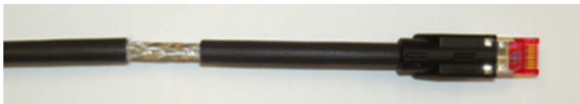
Fig. 10-12: Foil shield removed
