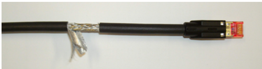
Fig. 10-11: Foil shield of the CDI cable
