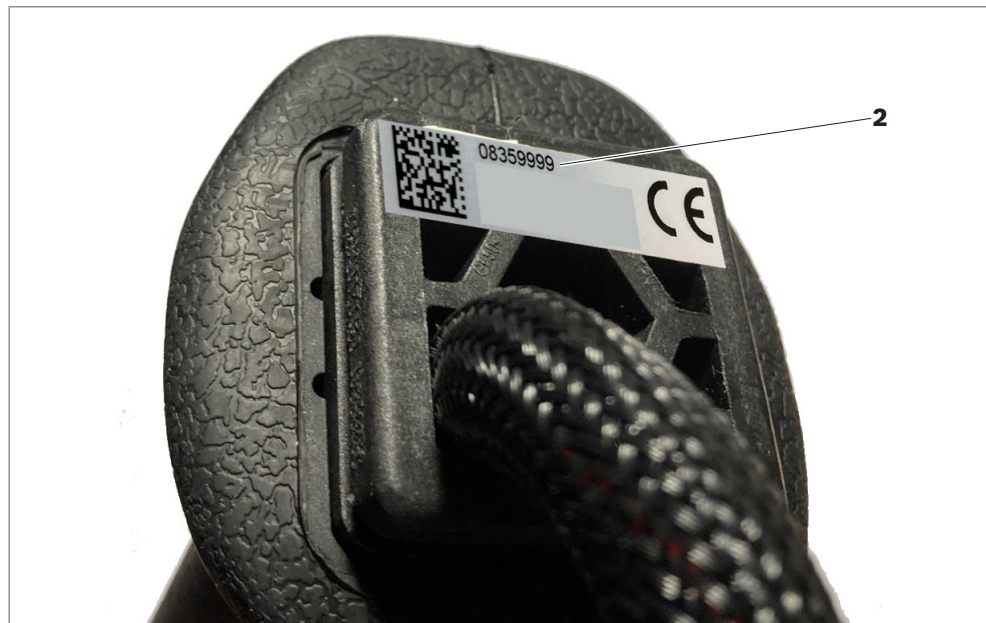
Fig. 3: Material number on sticker on the control grip
