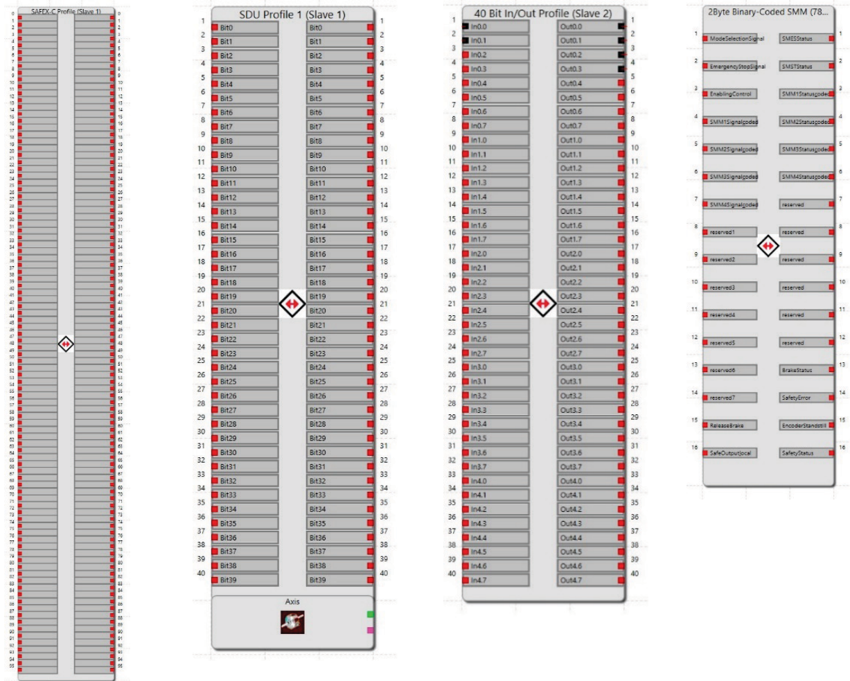
Fig. 82 Slave profiles (f.l.t.r.): SAFEX-C Slave profile, SDU profile, 40 Bit In/Out profile, 2 Byte Binary-Coded SMM
