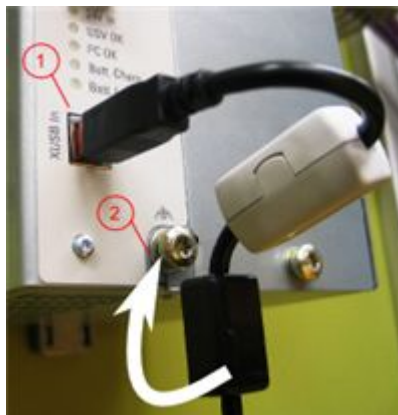
Fig. 10-6: Attaching the USB cable to the functional earth ground of the UPS
