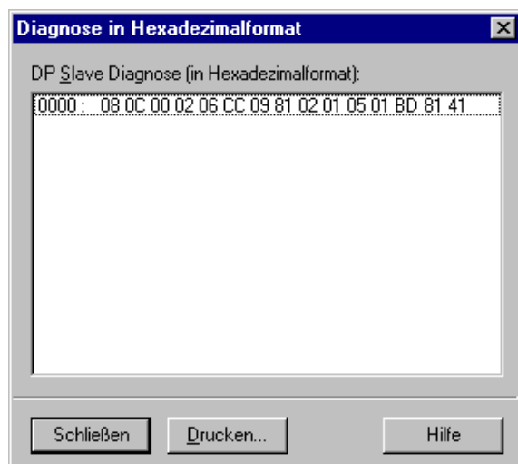
Fig. 4-25 I/O error on terminal 2 in status PDU format
