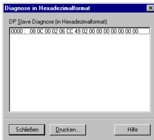
Fig.4-27 Peripheral fault on terminal 2 in "ID-specific diagnostic format"
