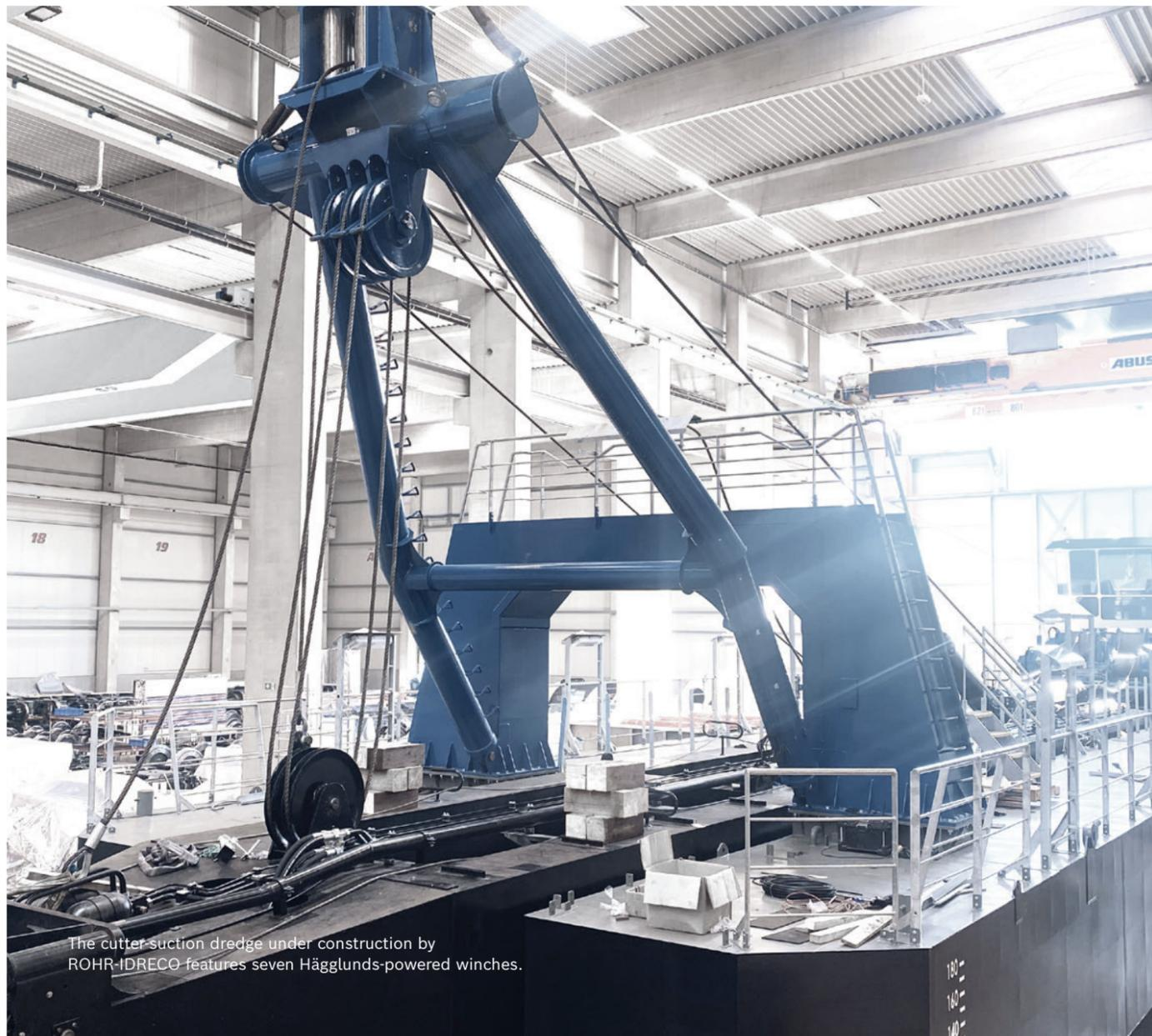
The cutter-suction dredger under construction by ROHR-IDRECO features seven Hägglunds-powered winches.
