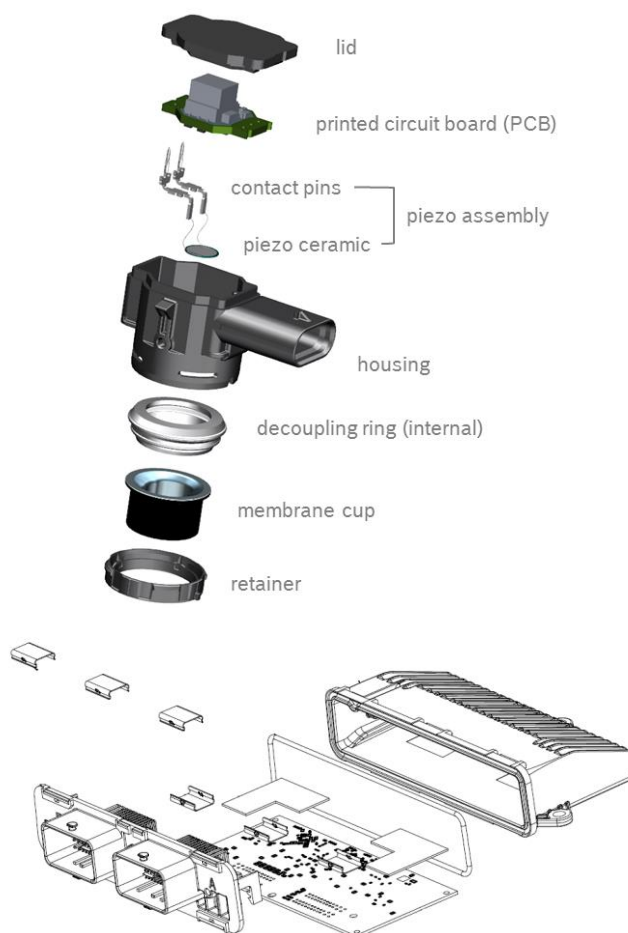
Figure 2 USS Sensor 6.5 with radial connector and ECU exploded view (not binding illustration)
