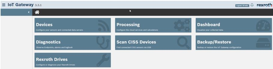
**Fig. 4-4:** The tiles show the basic functions enabled in the basic setting. More functions can be enabled, added or removed. Make these changes in the "Bundles" and "Licensing" menu.
