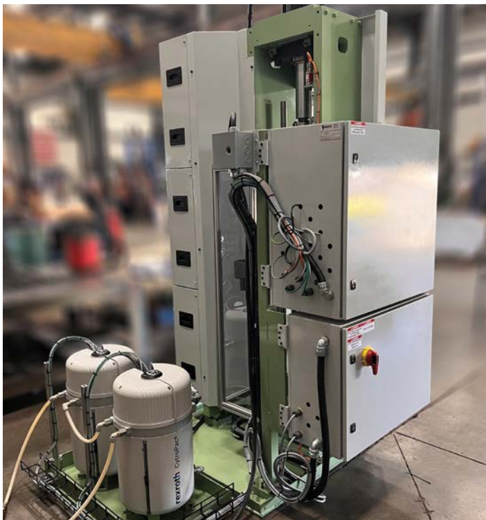
To deliver the necessary hydraulic flow within a small space, Bosch Rexroth devised a solution to link up two CytroPacs in a master/follower configuration.
