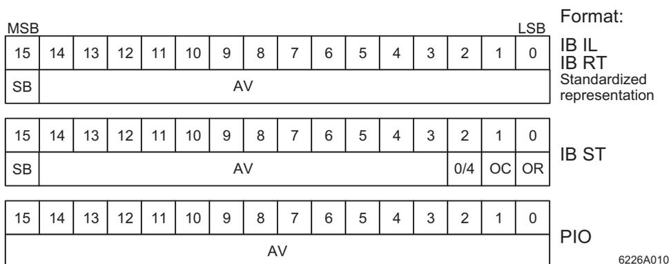
Fig. 9 Representation of the measured values in the different formats
