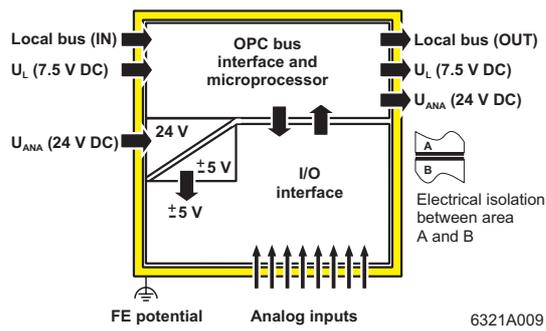
Fig. 3 Electrical isolation of the individual function areas
