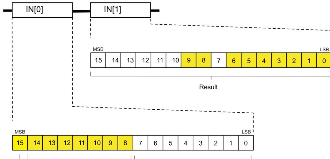
Fig. 8 Process data input words
