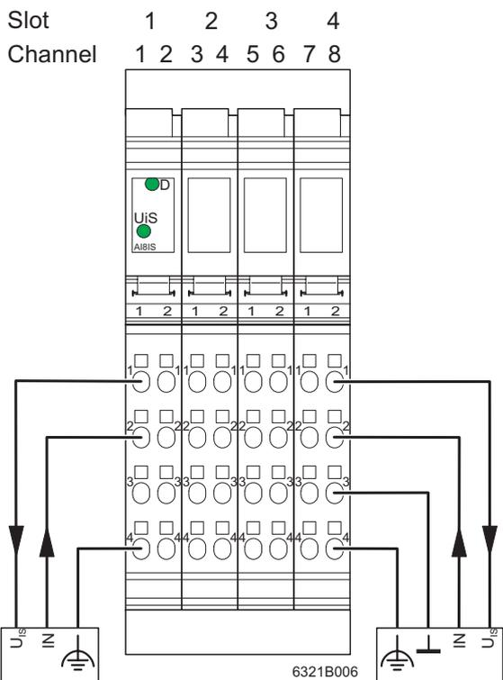
Fig. 5 Signals for the connection of passive sensors in 2 and 3-wire technology with shield connection
