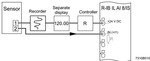
Fig. 6 Connection of several evaluating devices
