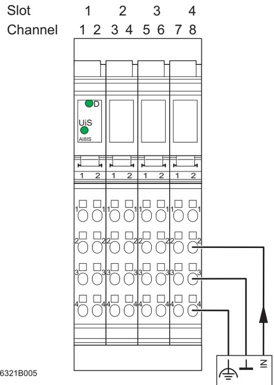
Fig. 4 Signals for the connection of active sensors in 2-wire technology with shield connection
