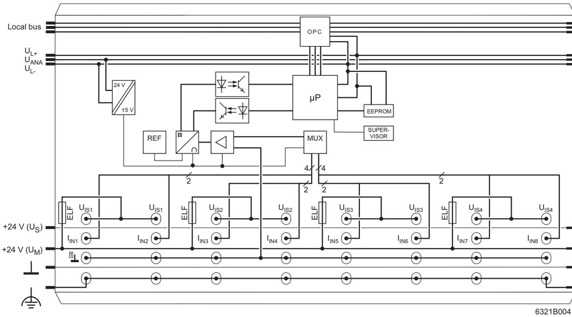
Fig. 2 Internal wiring of the terminal points
